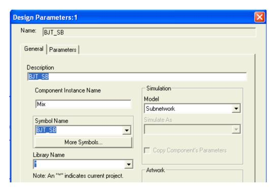
5. If you want to allow adjustable parameters from outside the subnetwork, use the Parameters menu tab. This is useful when you want to sweep some parameter that is inside the subnetwork. In this example, 4 parameters are declared to be adjustable. Their values are given a default, but can be specified again outside the model in the schematic where it is being used.
