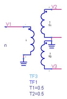
In ADS, the ideal center-tapped transformer is the TF3 icon in the components menu. For some unknown reason, however, the turns ratio is inverted from what you would expect to see. The primary side always is 1. The secondary windings are specified as 1/T1 and 1/T2. Hence, the T16-6T transformer, which has a total turns ratio of 4
